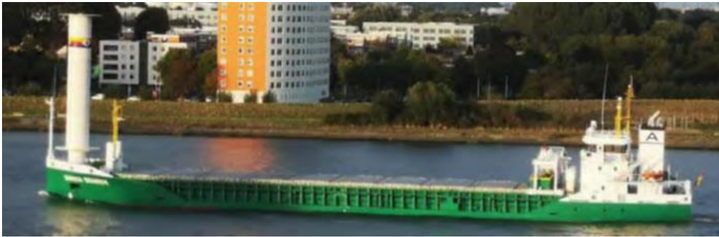
The " ANNIKA BRAREN " navigating the Oude Maas (NL) enroute Ronnskar (Sweden). The vessel, built in 2020, last year provided with an Wind-Assist Rotor at the foreship.
