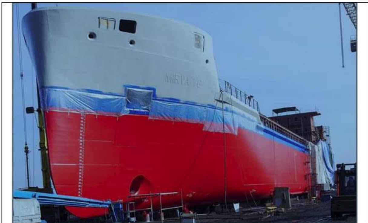
The finished hull of the MIRVA VG with two coats of Ecospeed. The inspector helps ensure that the applied coating will last the life of the vessel without the need for replacement.
